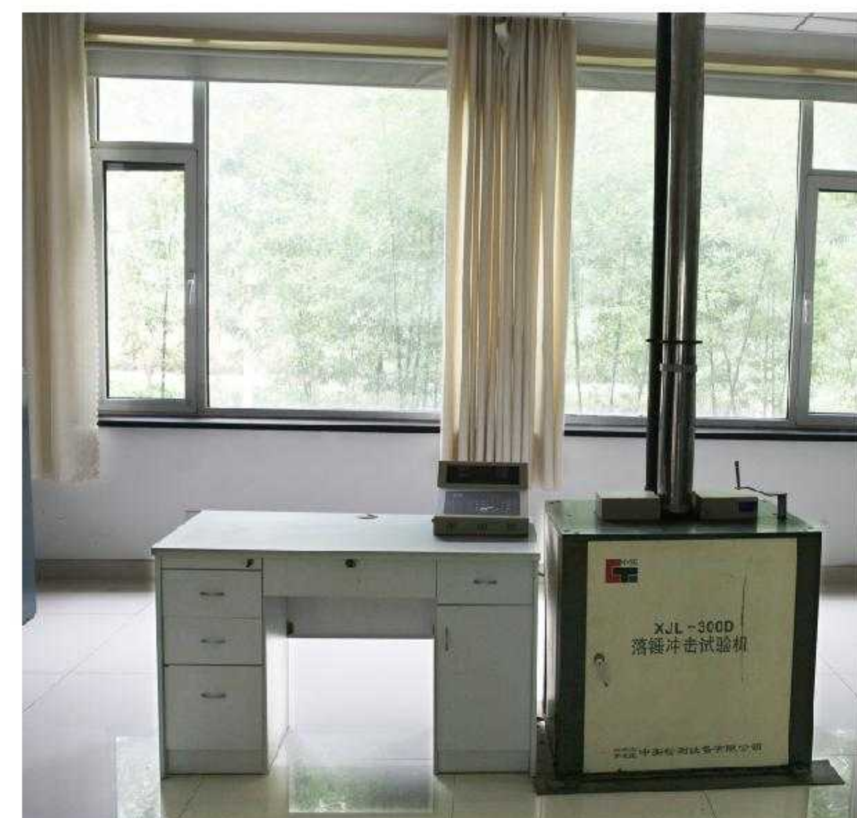
落锤冲击试验机 Drop hammer impact testing machine
