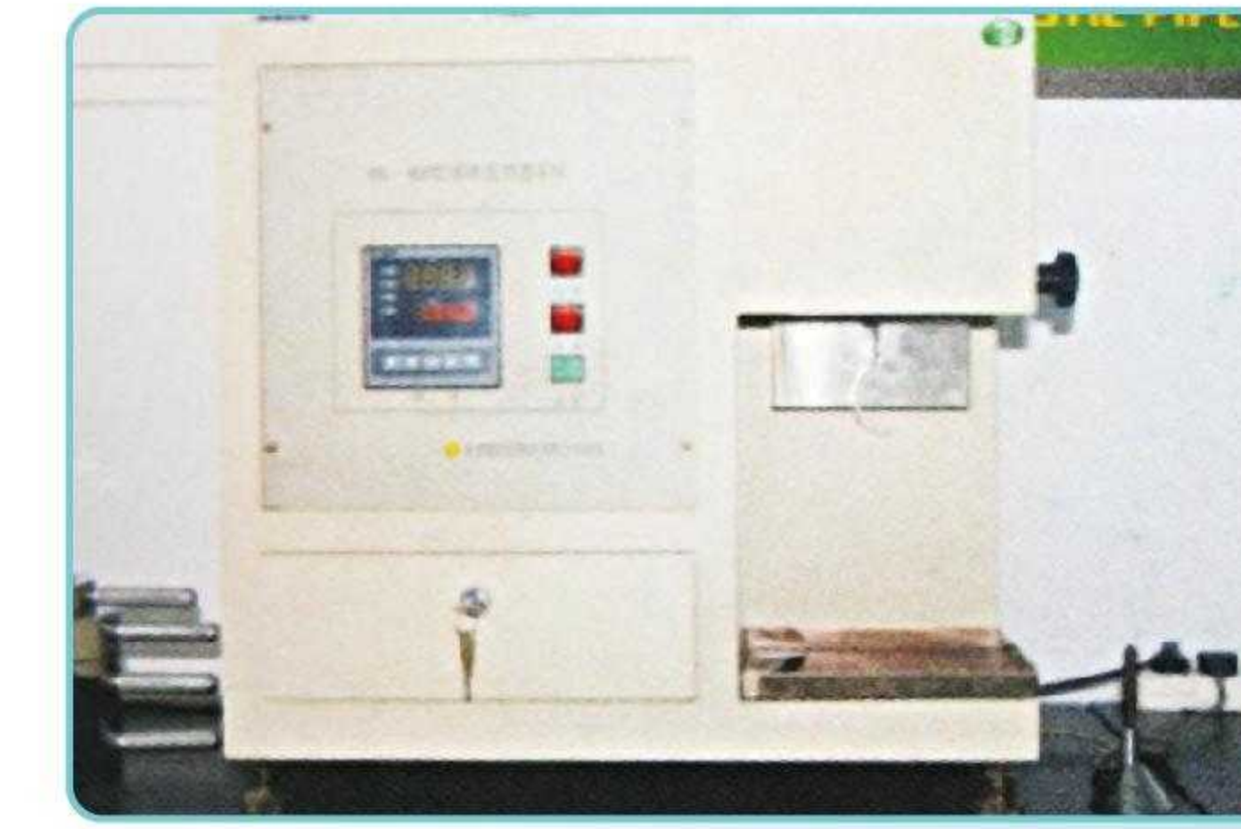
熔体流动速率仪 Melt flow rate meter
