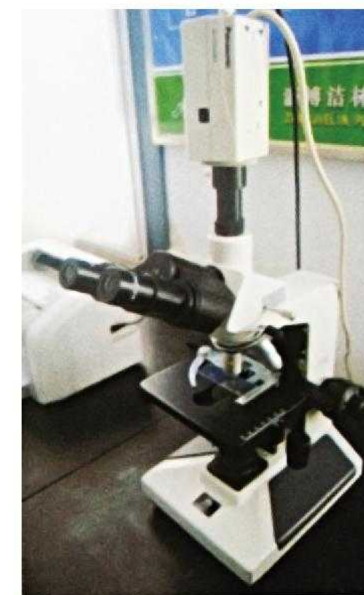
炭黑分散测试仪 Carbon black dispersion tester
