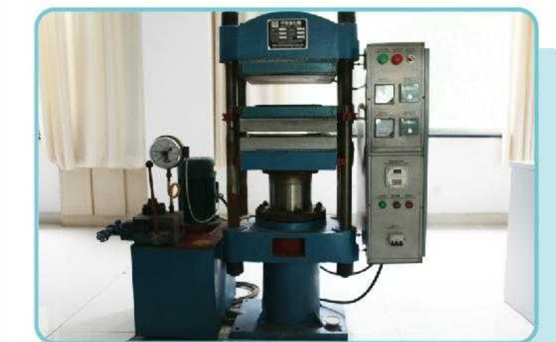
压缩复原试验机 Compression and recovery testing machine
