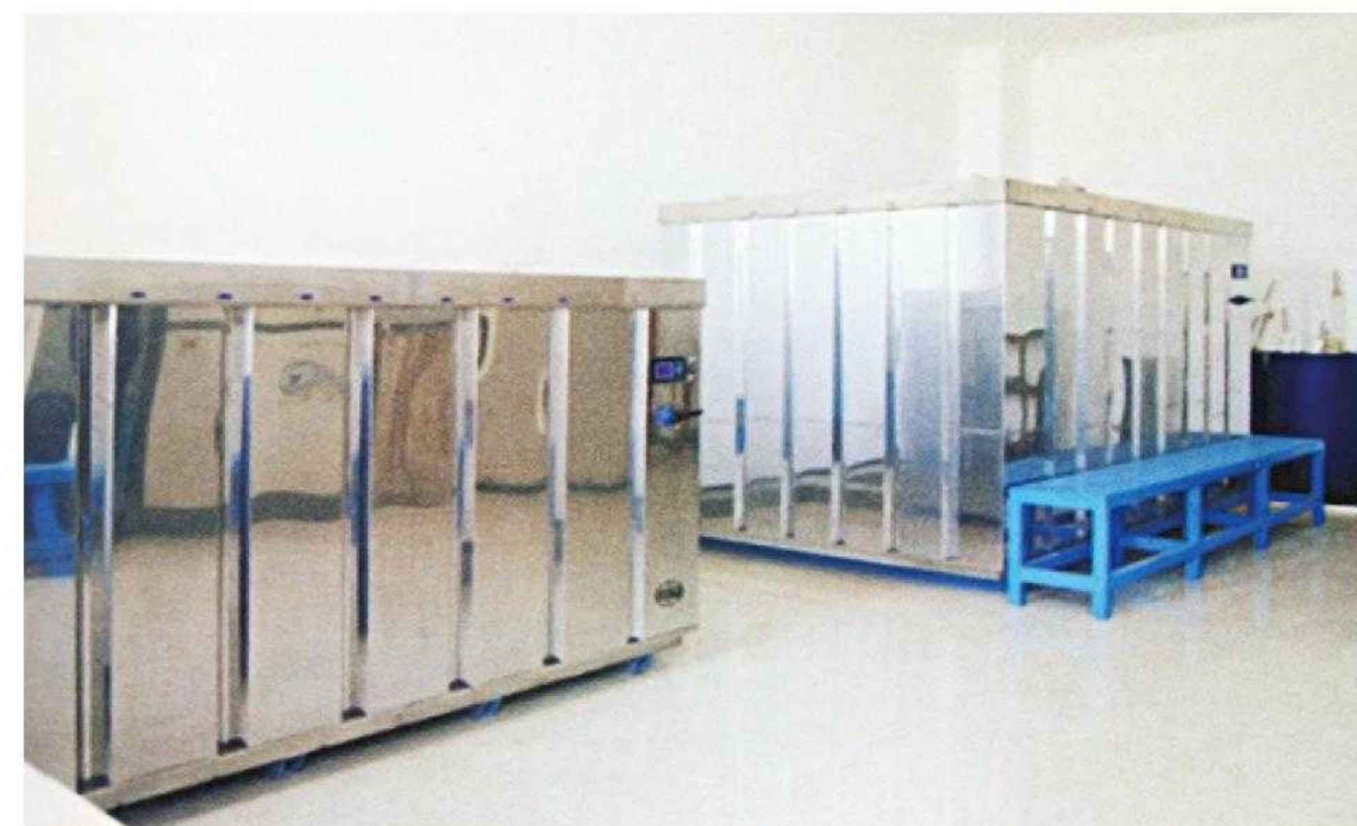
静液压试验水箱 Hydrostatic test tank
