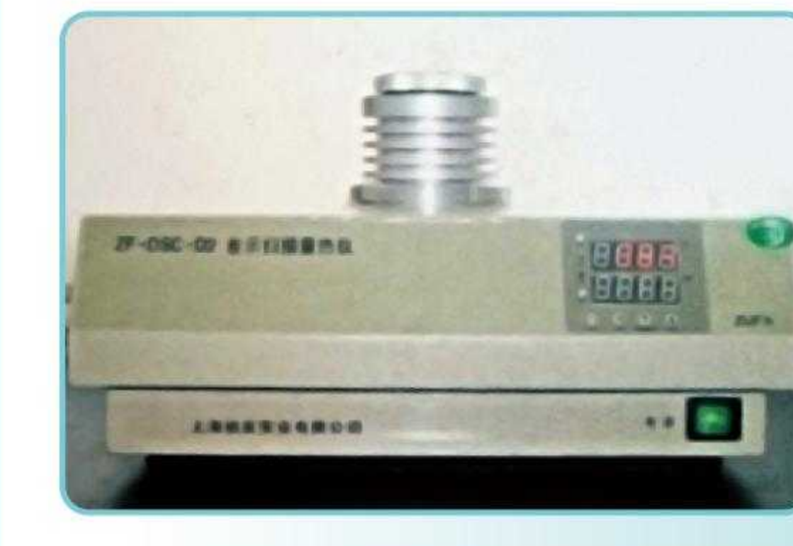
差示扫描量热仪 Differential scanning calorimeter
